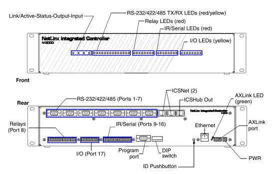
FIG. 4 NI-3000 front and rear panel components
